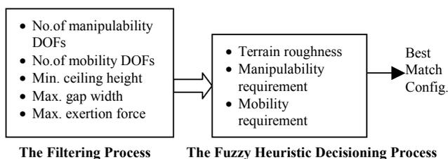
Fig 10. The configuration selection architecture
