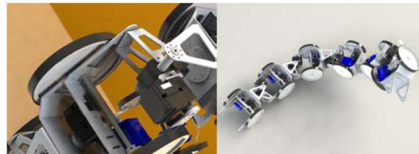
Fig. 1. CAD model of the modular snake robot.
