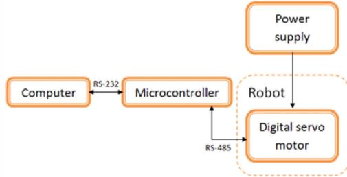
Fig. 2. System design of the modular snake robot.
