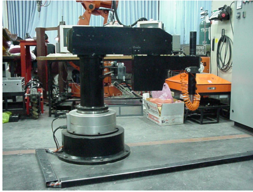
Fig. 2. SCARA robot manipulator used in experiment
