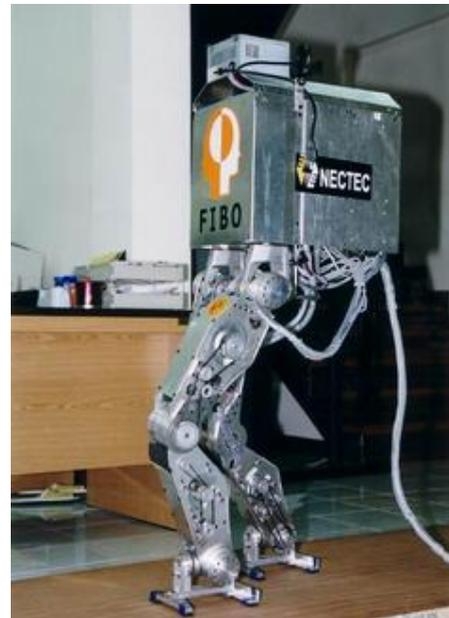
**Figure 1.** A first prototype of a two-legged walking robot.
