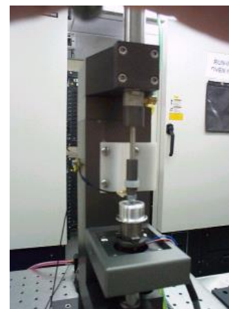
Figure 1 Vibration Measuring System for Spindle Motors
