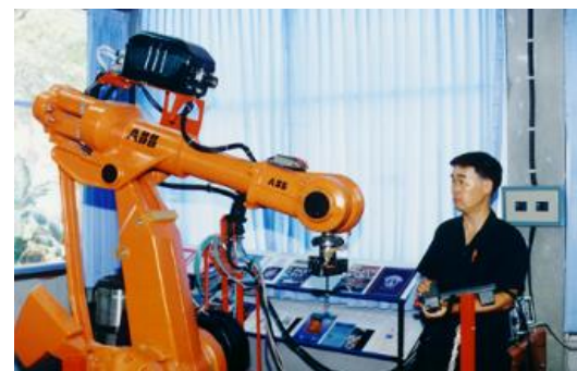
Figure 1 An industrial robot connected with a FIBO force sensor.
