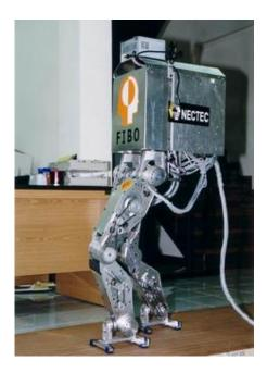
**Figure 1.** A first prototype of a two-legged walking robot.
