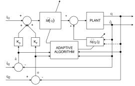
Figure 2 A block diagram indicating the controller and dynamic model of manipulator
