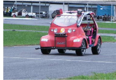
Fig.3. The experimental vehicle with three GPS receivers, the steering encoder and the rear wheel encoder.
