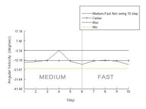
Fig. 7 Graph of the angular velocity during the transition from medium to fast walking gait with no swing arm (experiment 7).
