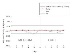
Fig. 10 Graph of the angular velocity during the transition from medium to fast walking gait with no swing arm in medium and swing arm in fast (experiment 10).
