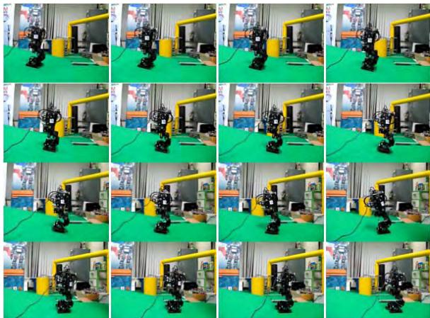
Fig. 11 Sequence of successive frames extracted from the video showing the robot when walking up on the inclined plane that changed from -10 to 0 degrees successfully.
