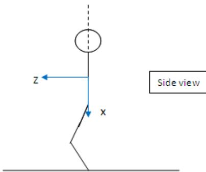
Fig. 2 Body angle calculation from 2-axis accelerometer
