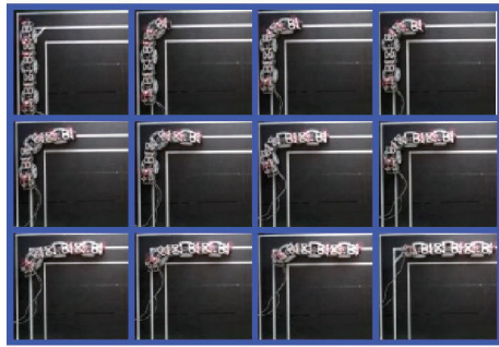
Fig.18. L-shape turning gait with varied driving speed
