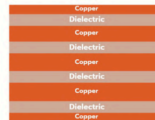
Proposed Thin-Dielectric Stacking
